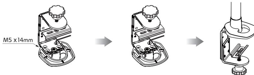
**Step 6** Stick EVA cushion to mount bottom. Mount assembly is completed for installation onto desk.
