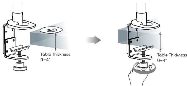
**Step 7** Install Mount with Swivel Arm, Spring Arm, and Monitor Bracket.
